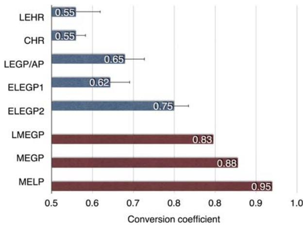
**Fig. 2** Conversion coefficients for various collimators
